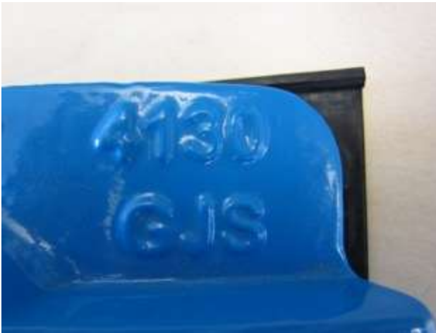
Material designation GJS cast on to body
