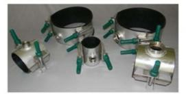
The CT Tapping Saddle is made from 316 Stainless Steel and is design for permanent tapping off take connections, on pressure (DI, CI, AC, MS) and non-pressure pipe systems. Host pipe sizes from DN80mm upwards, that require a permanent BSP tapping, 15mm, 20mm, 25mm, 32mm, 40mm or 50mm sizes available.
