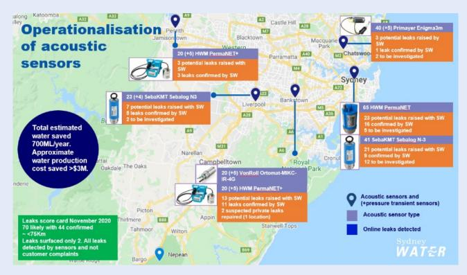
FIGURE 44 Online leak sensing map of acoustic sensors deployed across five CBD areas in Greater Sydney
